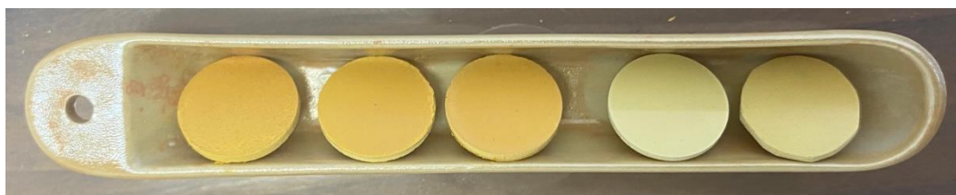
Figure 2.39: 13 mm \text{Bi}_{1-x}\text{Ln}_x\text{O}_{1.5} pellets in a boat before sintering at 750 °C for 12 hours.
