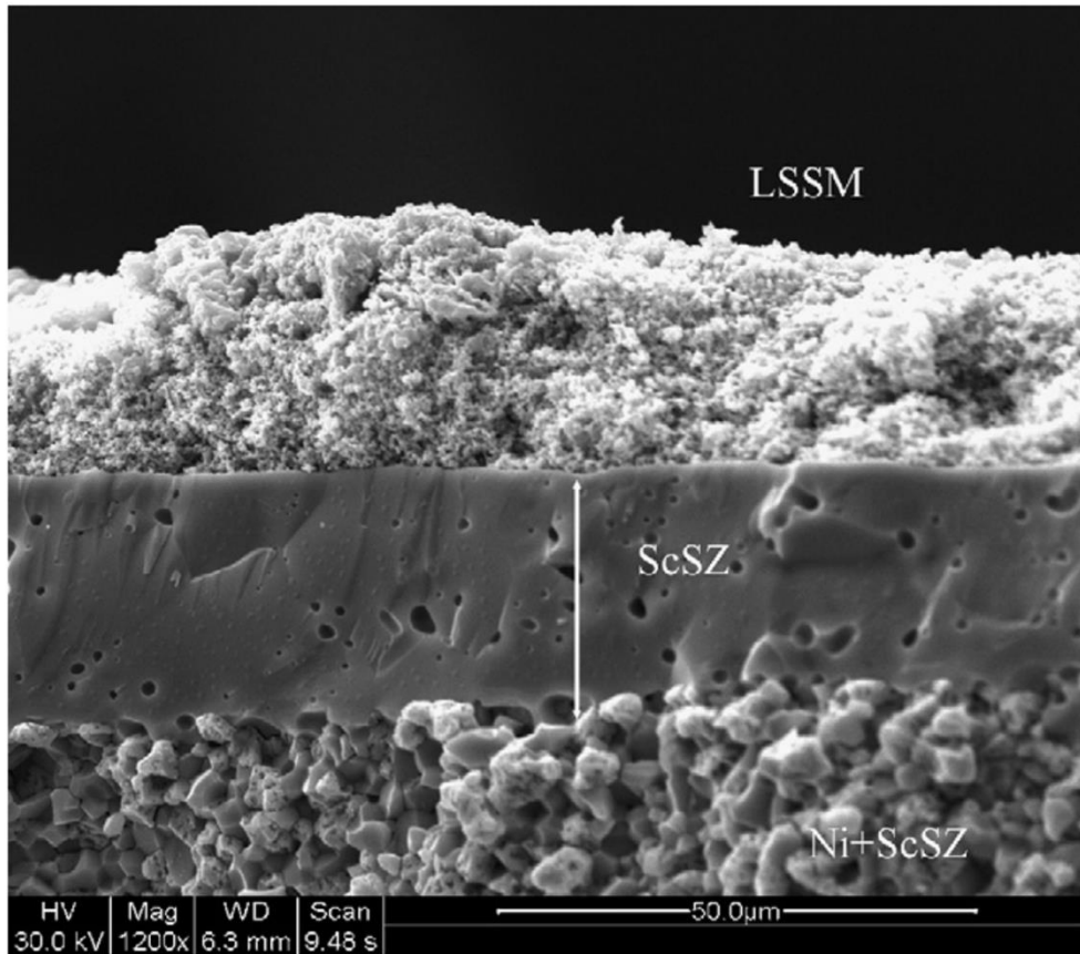
Figure 1.7: SEM image showing the cross section of a Scandium stabilized zirconia (ScSZ) and Ni supported film, ScSZ electrolyte, and Lanthanum strontium scandium manganate (LSSM) cathode of a SOFC. 33
