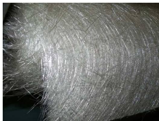
Figure 3.3; Glass fibre chopped strand mats, 350 g/m 2
