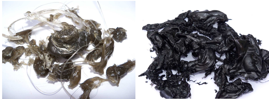
Figure 3.2: MWCNT reinforced polypropylene matrix: 0.1% MWCNT-PP and 1.25% MWCNT-PP
