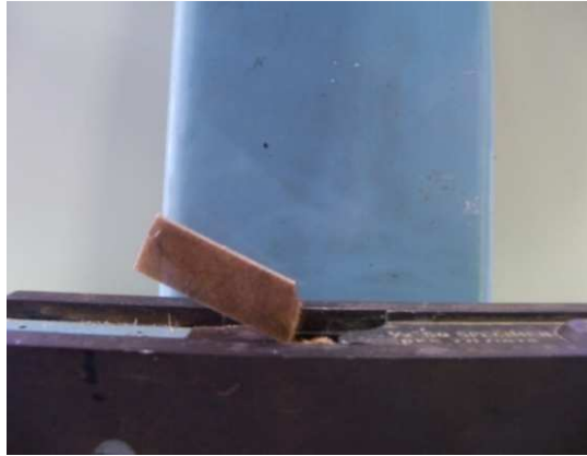
Figure 4.15: Kenaf/PP specimen under impact load
