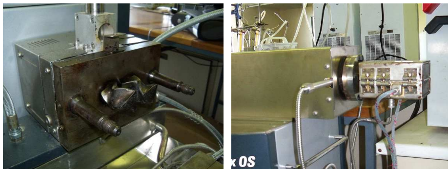
Figure 3.37: Double screws and extrusion die
