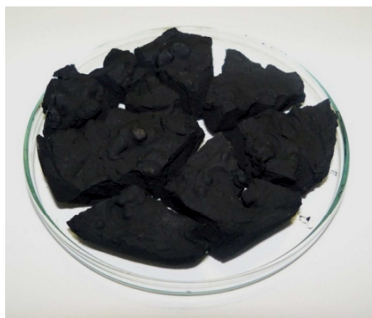
Figure 3.16: Filtrate of acid-silane treated MWCNTs
