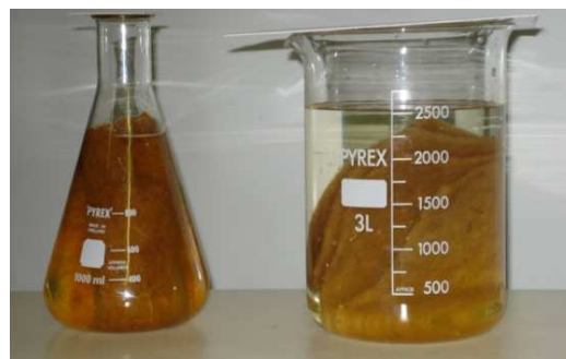
Figure 3.8: Alkali and alkali-silane treated of kenaf mats
