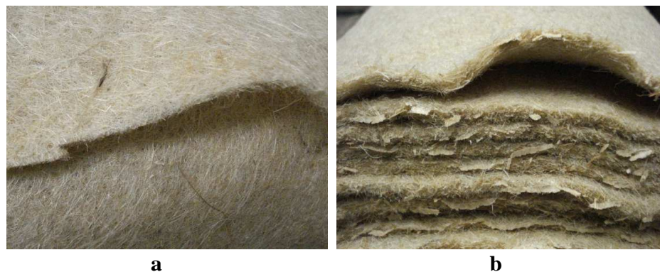
Figure 3.5: Kenaf fibres: (a) 125 g/m 2 mat, (b) 350 g/m 2 mats
