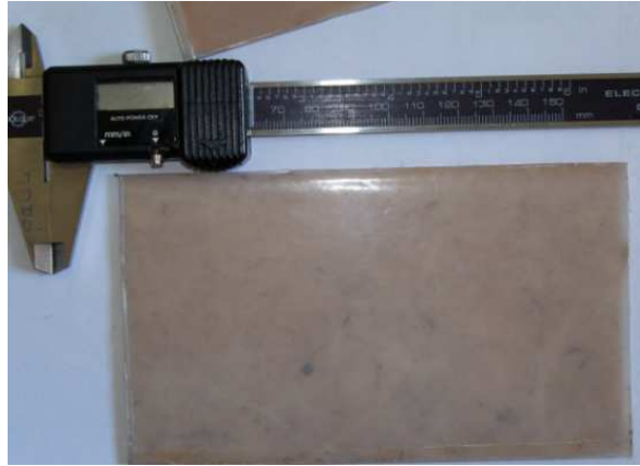
Figure 3.34: Kenaf/PP composite plates
