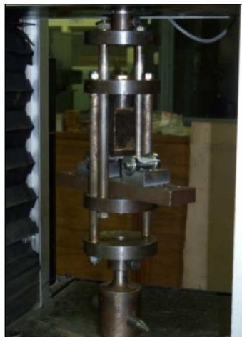
Figure 4.2: Flexural test set up on Lloyd MX100
