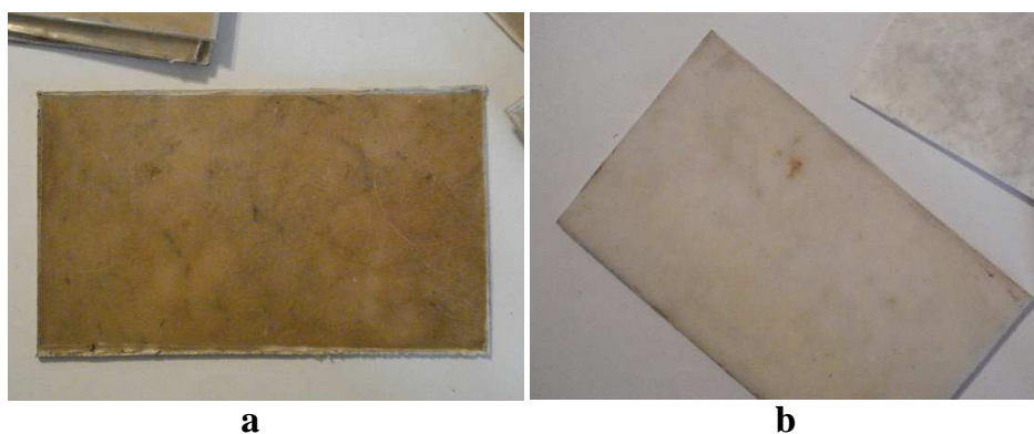
Figure 4.17: Test specimens: kenaf/PP and glass/PP composites
