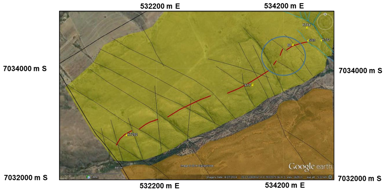
Figure 5.7. Knotted quartzite horizon (red line) shown in Figure 5.6 is displaced by generally northwest-trending D4 fault sets (blue circle) in the Turffontein Subgroup. Samples collected from the horizon are also plotted.
