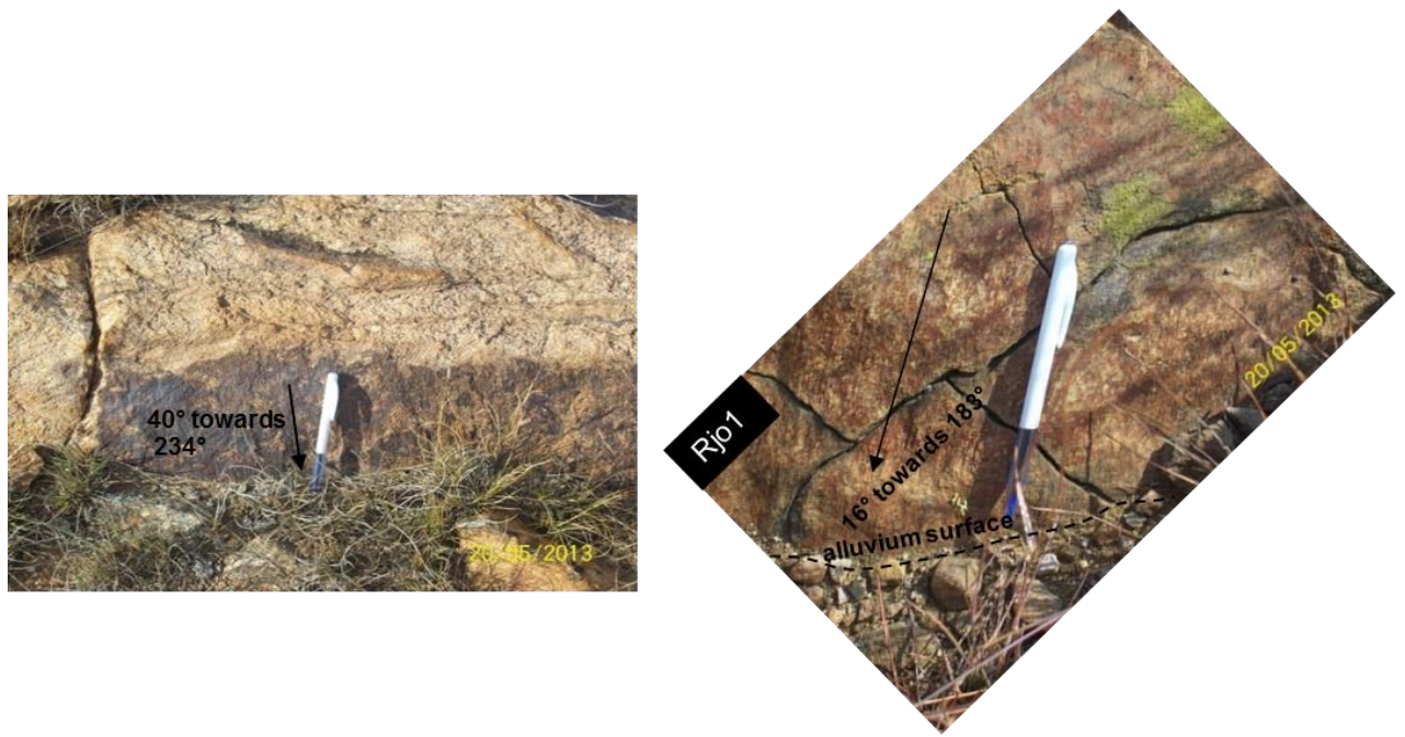
Figure 5.21. Striated bedding planes indicative of dip-slip (35 J 541884 m E, 7037457 m S; and 35 J 541789 m E, 7036718 m S).
