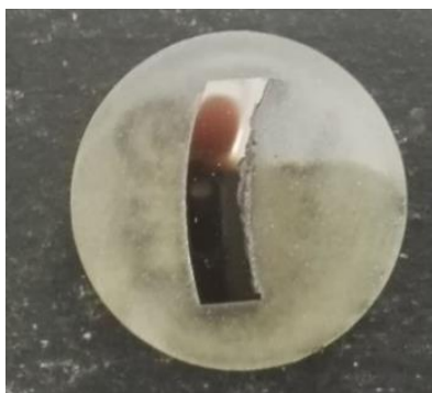
Figure 3.3: A cross section specimen of the tube prepared for QEMSCAN analysis, mounted in cold mounting resin, external surface with the fireside deposit on the left, and the internal surface (waterside) on the right.
