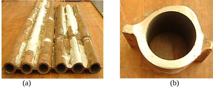
Figure A.5: Side wall tubing samples from Unit 4 of Station A, showing (a) fireside deposit and (b) wall thinning on the fireside.
