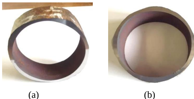
Figure A.7: Division wall tube sample from Unit 3 of Station B, showing (a) fireside deposit and (b) wall thinning on the fireside.
