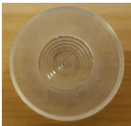
Figure 3.6: Sample holder for powder specimen to be analysed with XRD.
