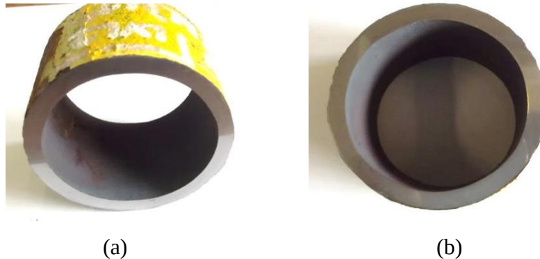
Figure A.6: Tubing samples from division wall of Unit 1 of Station B, showing (a) fireside deposit and (b) wall thinning on the fireside.
