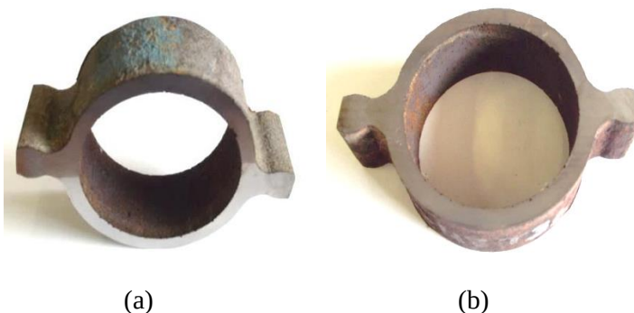
Figure A.8: Side wall tube sample from Unit 8 of Station B, showing (a) fireside deposit and (b) wall thinning on the fireside.
