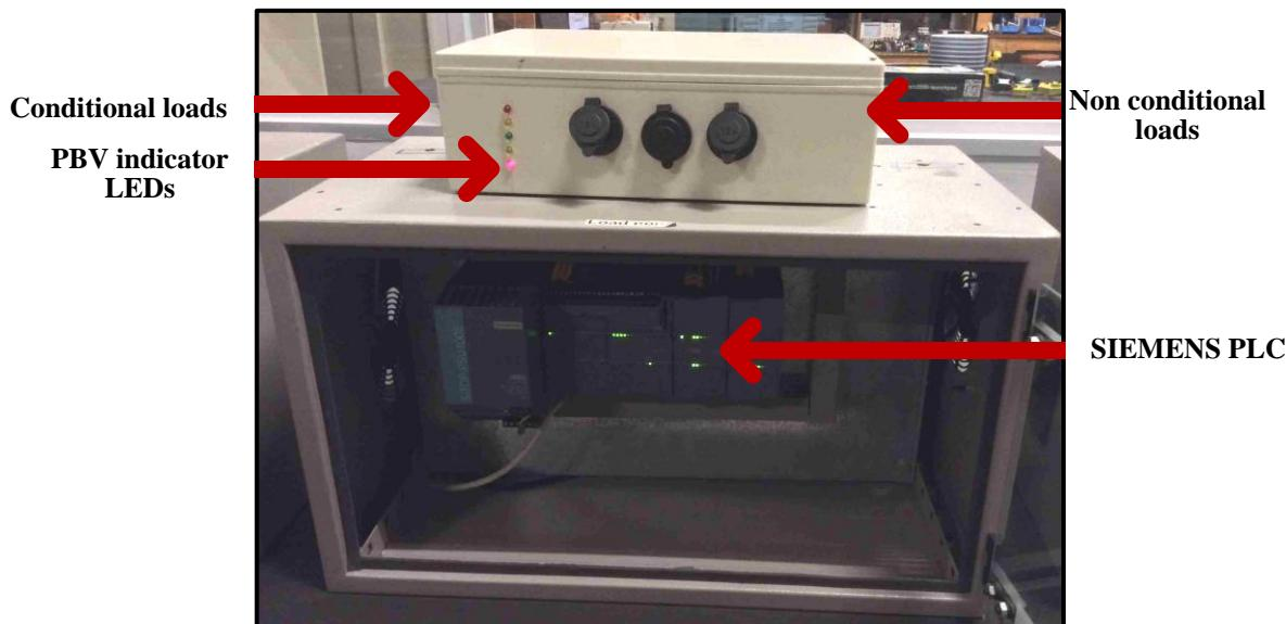
Figure 19: Load node picture
