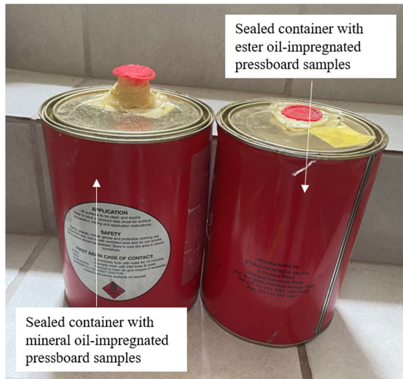
Figure 3-3: Oil Impregnated Pressboard Samples in Airtight Containers
