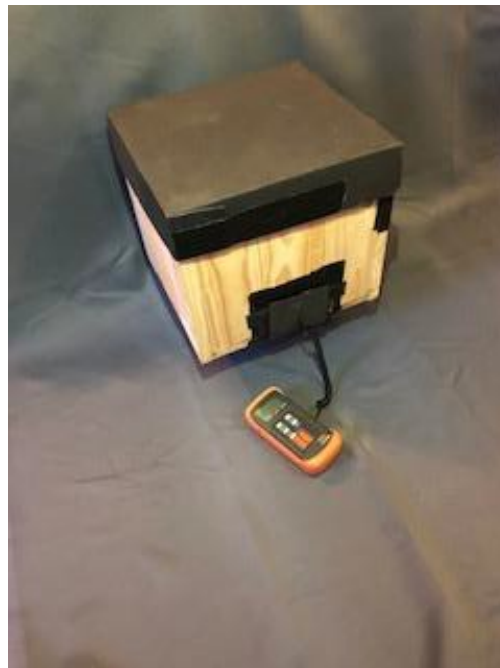
Portable dark box with laryngoscope and light sensor in place
