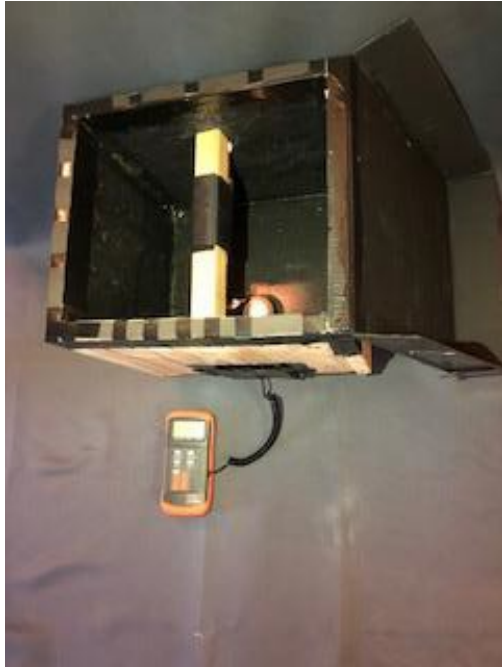
Portable dark box with laryngoscope and light sensor in place
