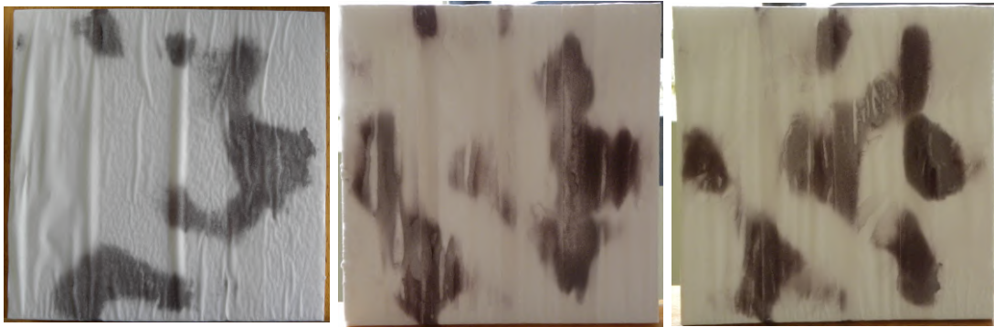
Figure 4.4: The near fields inside the microwave oven as shown on thermal paper.
