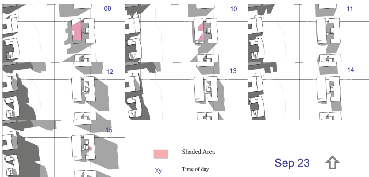
Figure 4.14: Building D – Medium density urban fabric. Detail of shadow study illustrating shadows (pink) from 9am – 3pm on 22 September.
