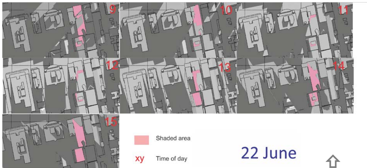
Figure 4.6: Building B – High density urban fabric. Detail of shadow study illustrating shadows (pink) from 9am – 3pm on 22 June.
