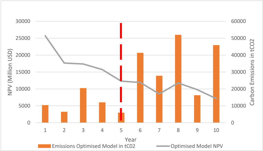
Figure 4.6 Optimised Model's NPV vs Carbon emissions over 10 years.
