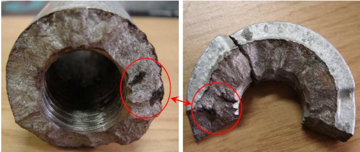
Figure 3.7 Dark stained areas found on the fracture surface (Calitz, 2008)
