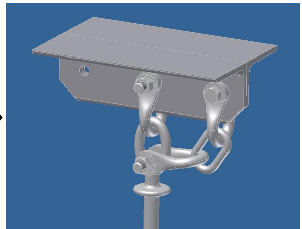
Figure F.4 Redundant assembly
