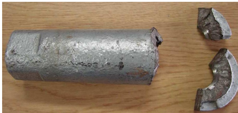
Figure 3.6 Failed ratchet nut (Calitz, 2008)
