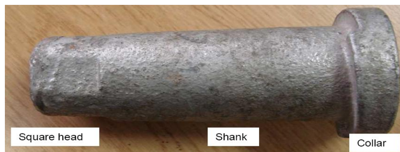
Figure 3.5 Descriptions used for the different sections of the ratchet nut (Calitz, 2008)
