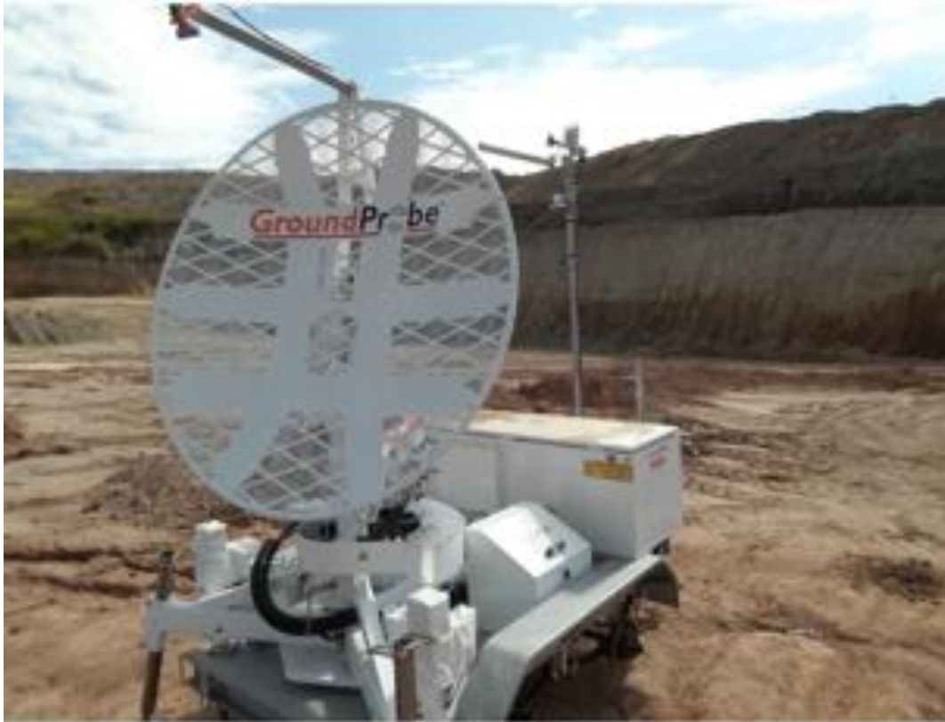
Figure 2-16: Slope stability radar image at COPF/D
