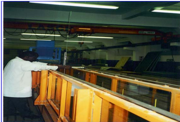
Figure 4.10: Flume section showing a vernier scale mounted on a movable rail gauge
