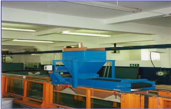
Figure 4.3: Sediment feeder mounted on the flume
