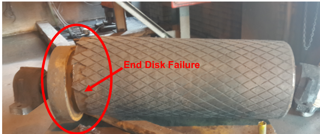
Figure 1.4: Pulley end disc failure
