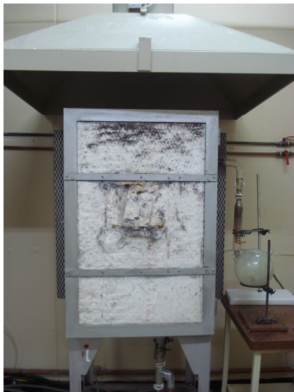
Figure 26: Furnace used for chlorination experiments
