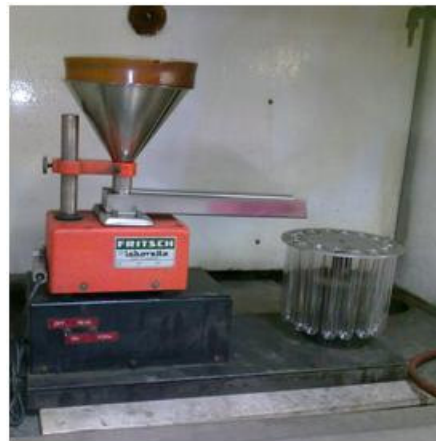
Figure 23: Rotary Splitter used for 2 nd and 3 rd stage sample splitting
