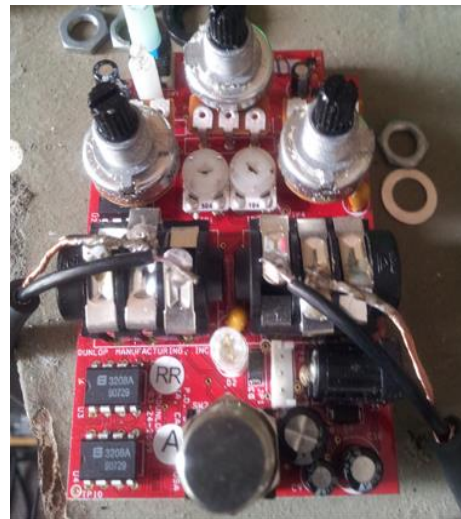
Modifying circuit boards so as to remain 'always on'
