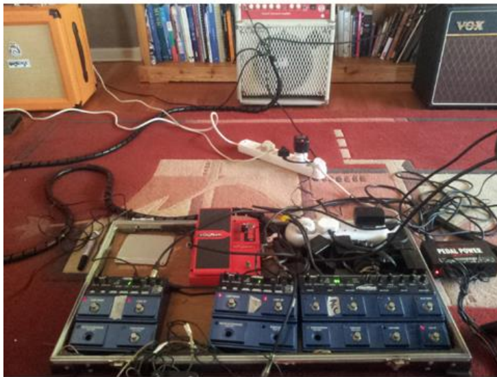
First testing of 3-way loop system on three amplifiers
