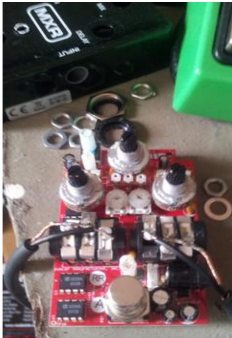
Modifying the MXR board to remain 'always on'
