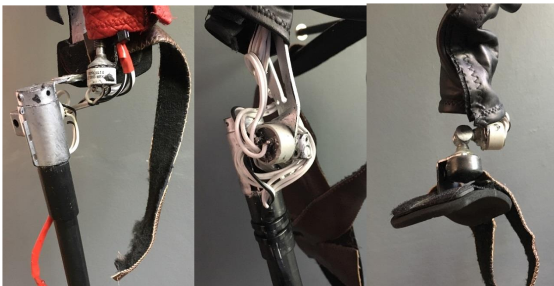
Figure 45: Exoskeleton elbow, shoulder and wrist joints.
