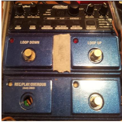
First loop station with REC/PLAY/OVERDUB switch removed
