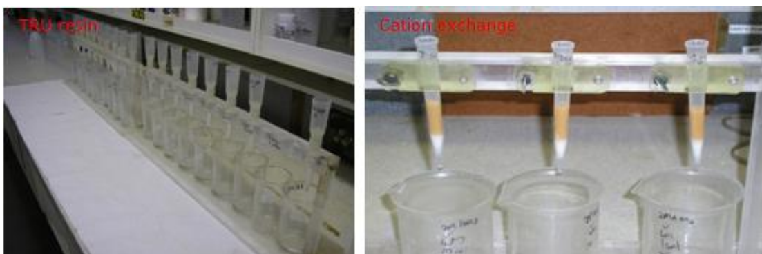
Figure 4-13: Separation of Uranium using extraction chromatography and cation exchange chromatography
