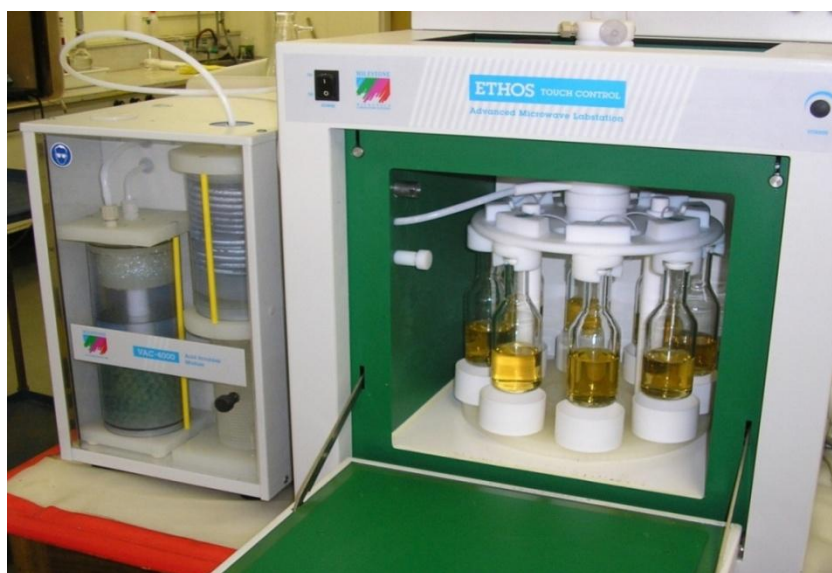
Figure 4-11: Using an open vessel microwave for digestion of fish
