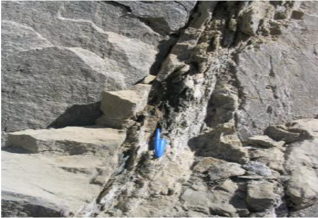
Figure 16: Steeply dipping shear zone, northern portion of the Phoenix pit. Source (SRK, 2006)
