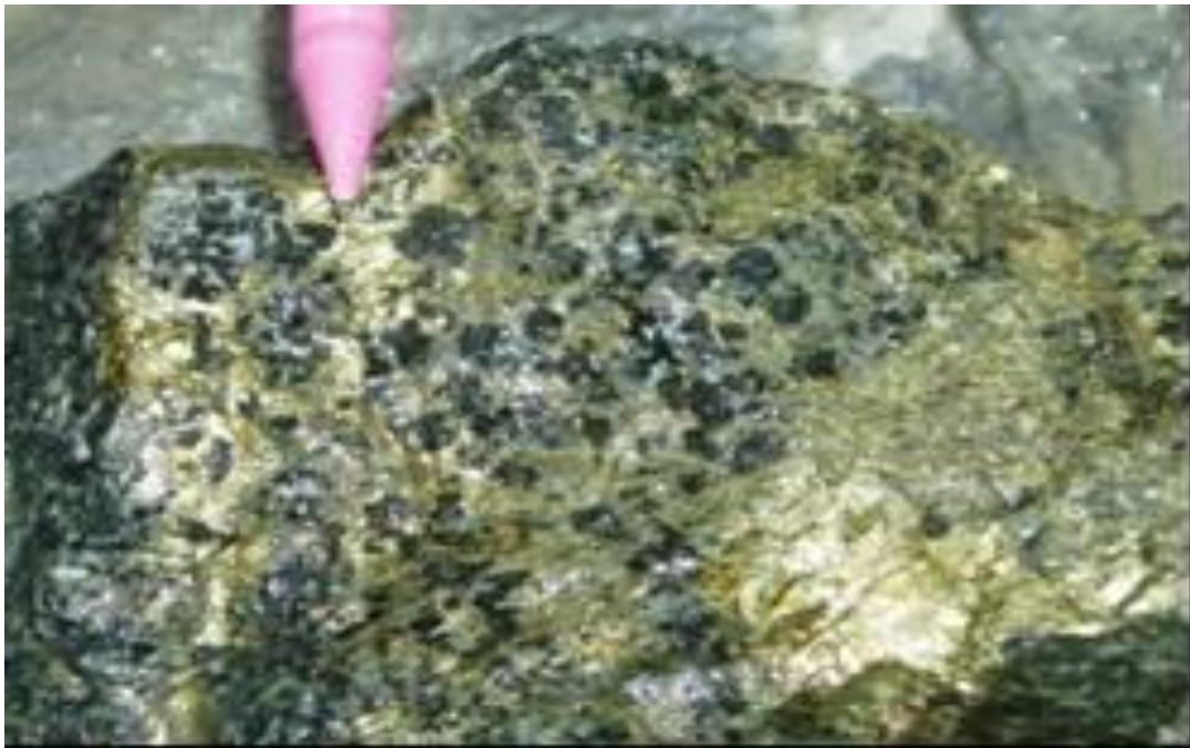
Figure 17: Semi-massive sulphide mineralization in pit metagabbro. Source (TWP, 2006)
