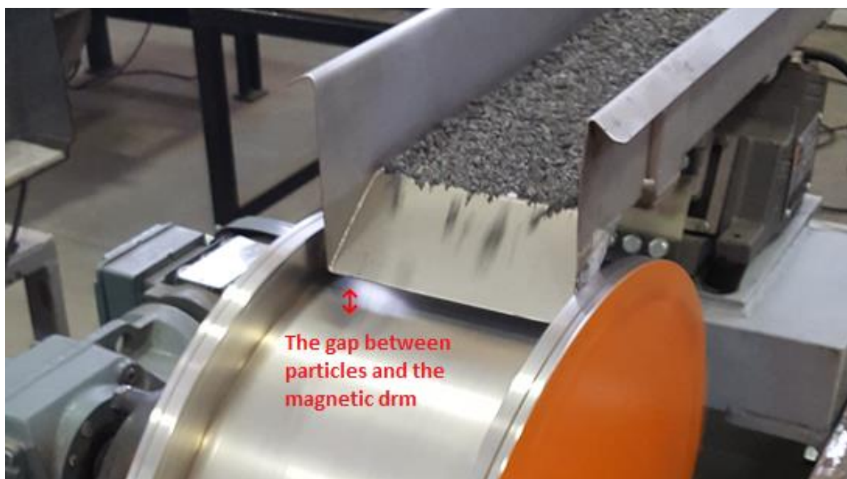
Figure 9.4: Distance between particles and magnetic drum
