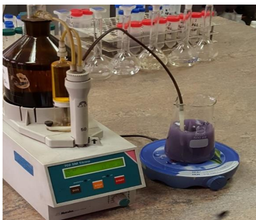
Figure 3.4: Set up to determine the total iron content by the titration technique
