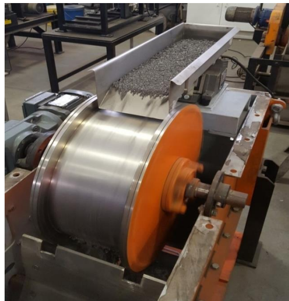
Figure 3.2: A dry magnetic drum separator
