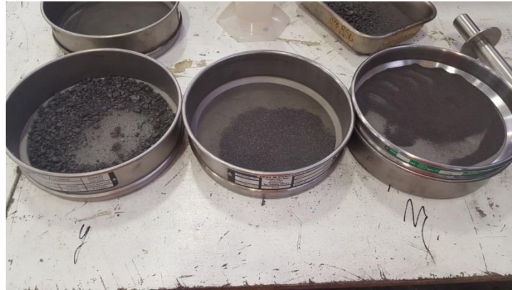
Figure 3.3: Visual appearance of different particle size classes in sieves
