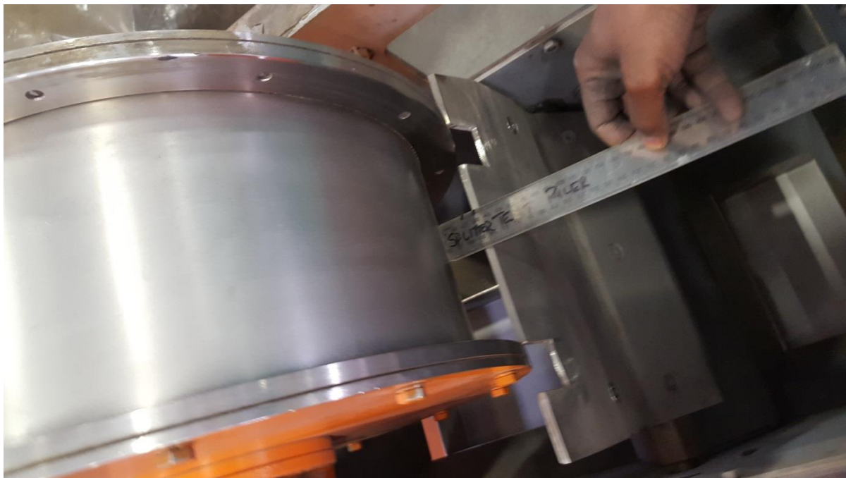
Figure 9.3: Magnetic drum –Splitter position
