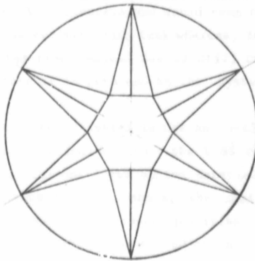
Figure 77. Plan view of cone with 6 triangular gutters.
