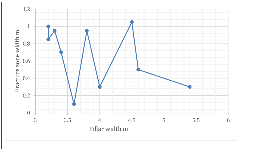
Figure 9.3.3_3. Width of zone between commencement of dog-earing and the pillar sidewall.
