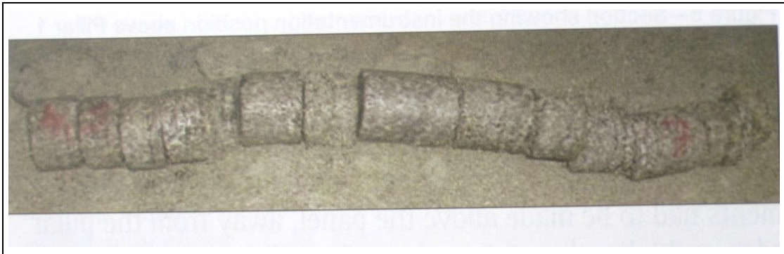
Figure 0_1 Core discing of borehole core obtained from above a Pillar - (Watson et al, 2007)
