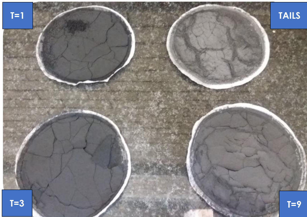
Figure 5.10 Flotation Products at Diesel Dosage 14g/kg Coal
