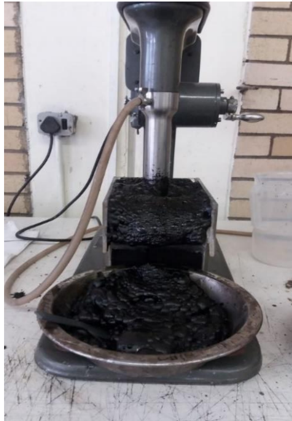
Figure 5.9 Froth Flotation of Low-Grade Coal Sample using a Denver Machine
