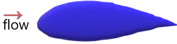
Figure 3.6: Airfoil shape has the smallest C_d
