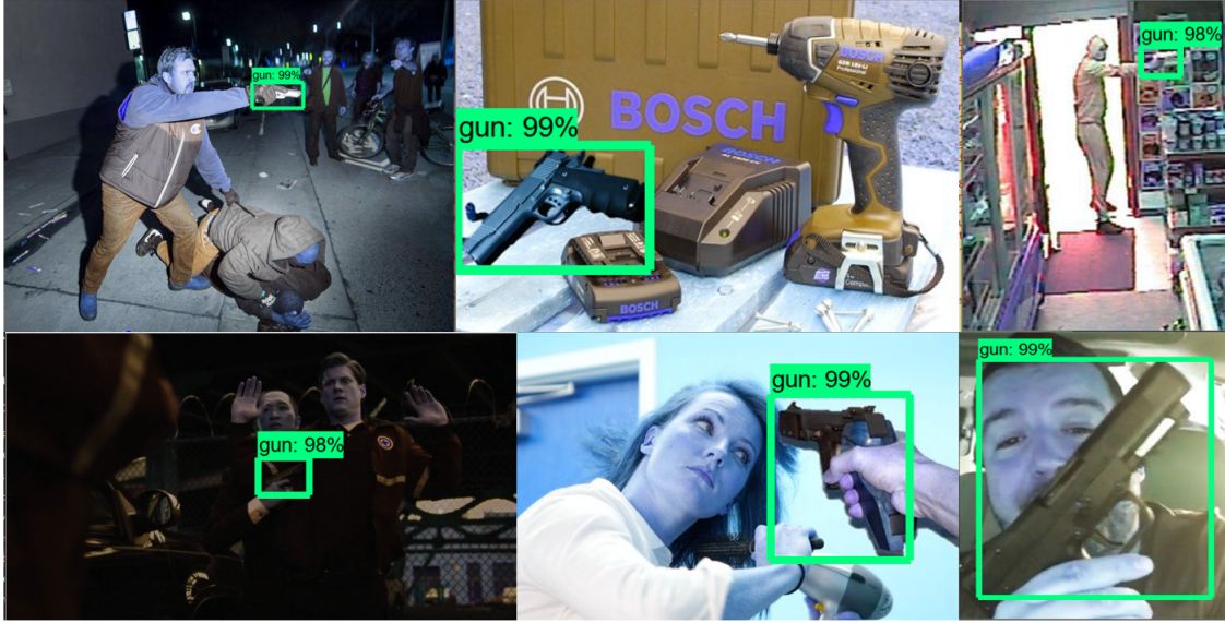
Figure 6.5: RFCN firearm detection samples taken from results obtained by Group B. In these images, all guns were detected accurately. The confidence score of the top-right and bottom-left images is lower than those scored in other images due to the small size of the firearms. This shows that RFCN is able to better process larger sized firearms than those at a small scale.
