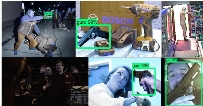
Figure 6.1: SSD firearm detection samples from Group B classifier results. SSD is easily able to detect firearms that contrast with background colours. The top-right and bottom-left images each contain a firearm which are small in size and are coloured similarly to its background. This creates a blending effect which caused the SSD classifier to predict a FN.
