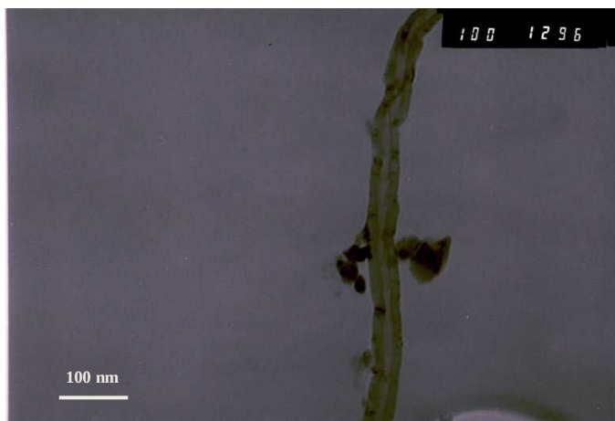
Figure 4. 15: CNT produced at 850°C using Mischmetal catalyst.
