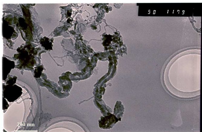
Figure 4. 13: CNTs produced at 750°C using Lanthanum-Nickel alloy.
