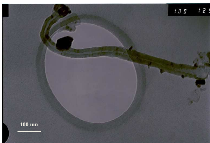
Figure 4. 16: CNT not fully formed.
