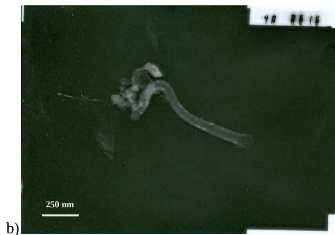
Figure 3: a) CNFs; b) possible CNT at 700°C using Lanthanum-Nickel catalyst.
