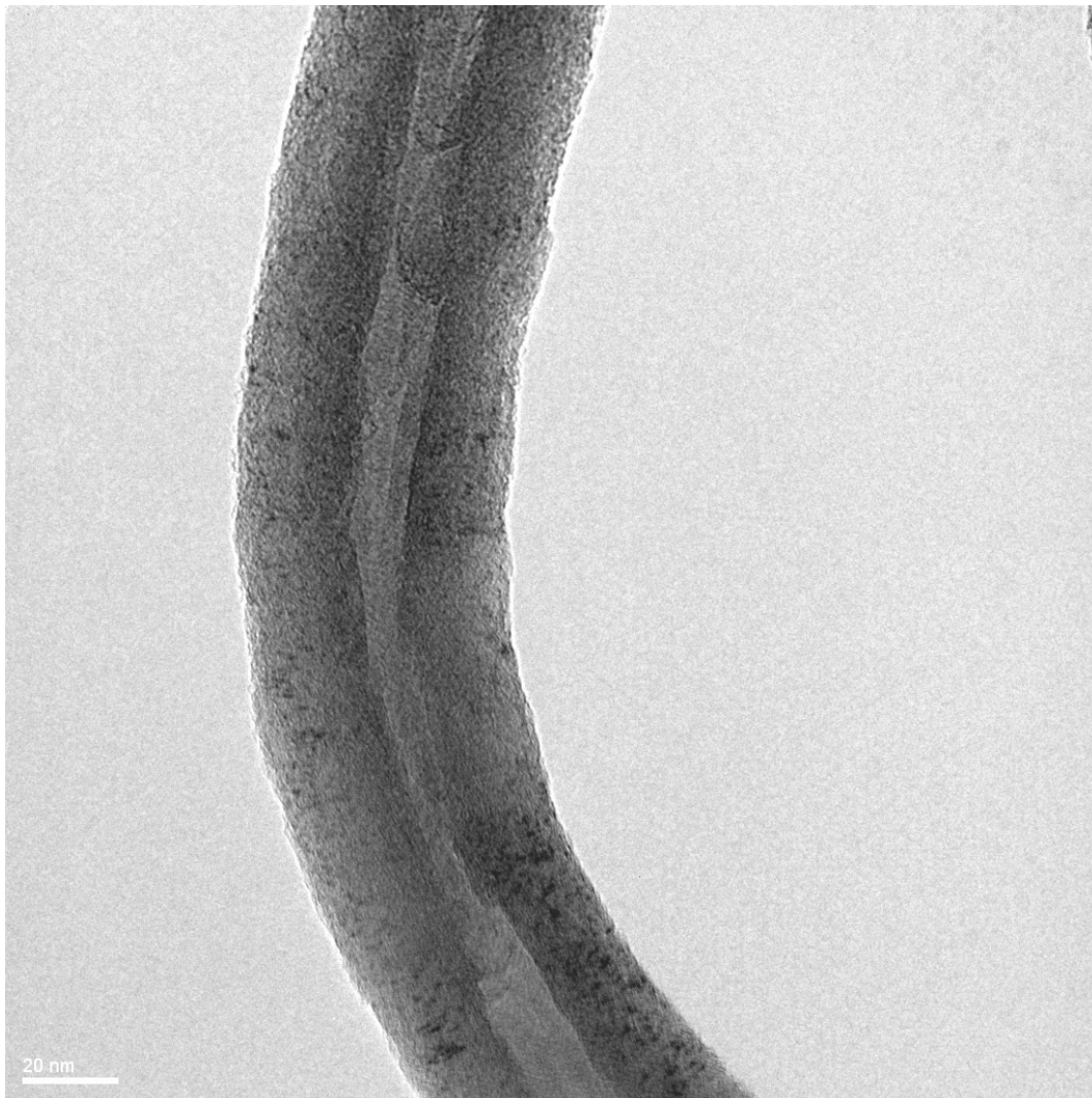
Figure 4. 12: HRTEM image of CNT produced at 650°C using Lanthanum-Nickel alloy.
