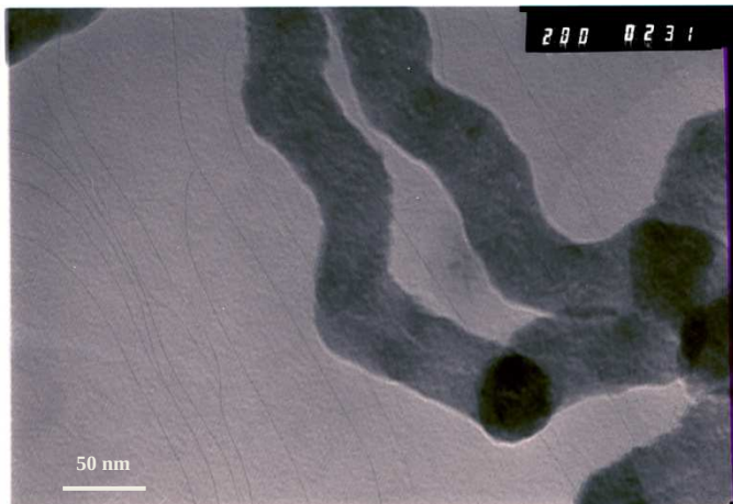
Figure 4. 3: TEM image of the CNF on the nickel catalyst.
