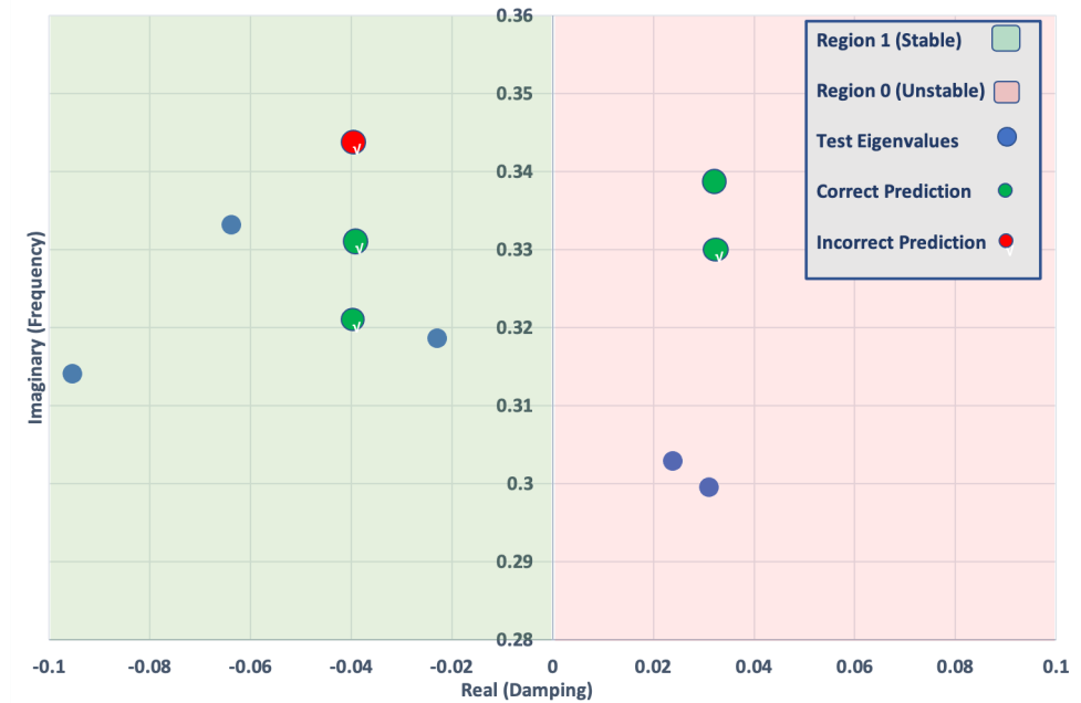
Figure 41: Eigenvalue plane showing the test eigenvalues and the predicted eigenvalues according their respective regions
