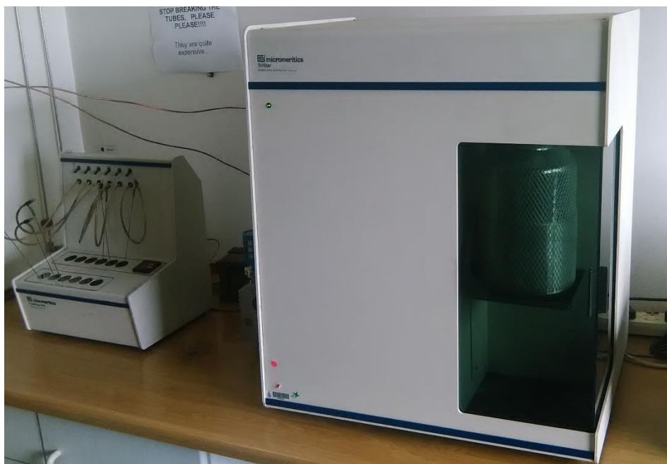
Figure 3. 6. Micromeritics Tristar Surface area and Porosity analyser.
