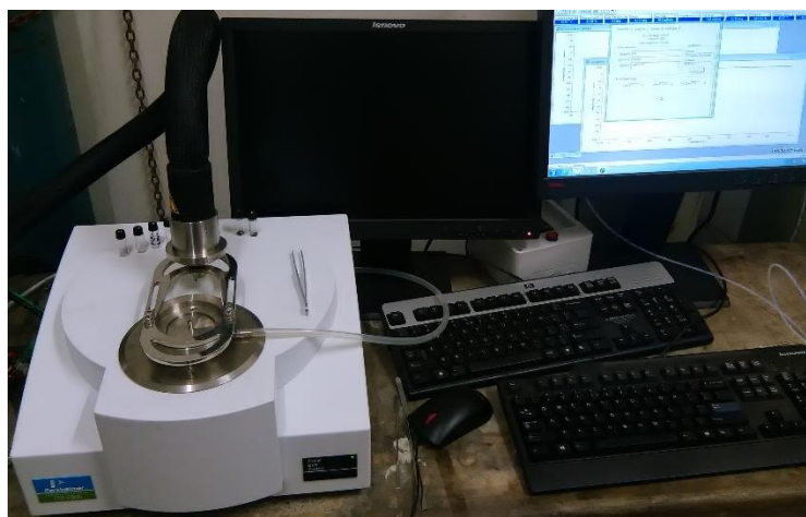
Figure 3. 7. Perkin Elmer STA 4000 Simultaneous Thermal Analyser.
