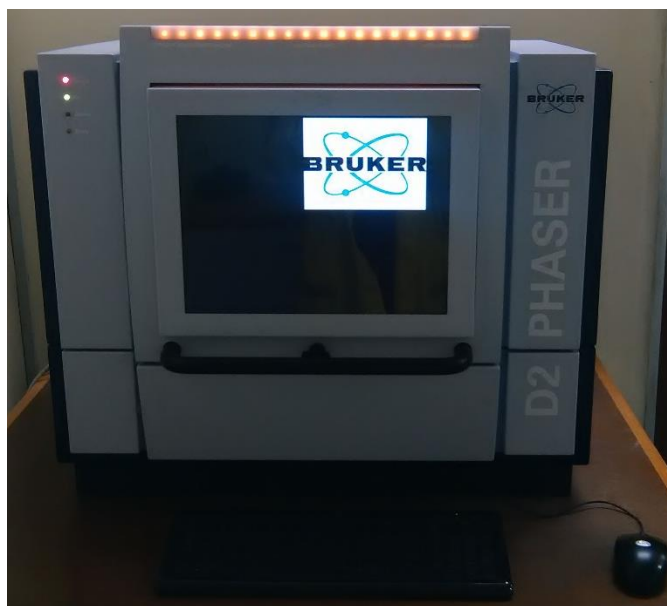
Figure 3. 3. Bruker D2 PHASER desktop powder X-ray diffractometer.
