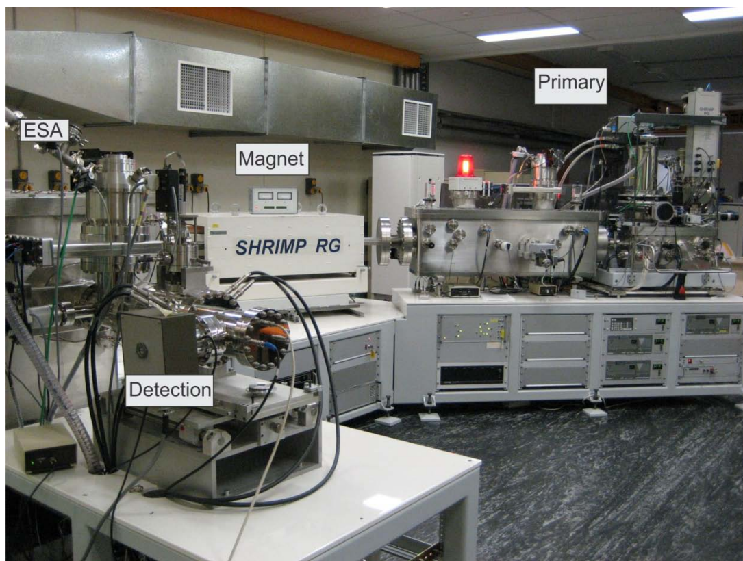
Figure 2.4: Photograph showing the configuration of the Reverse Geometry SHRIMP housed at the ANU (note the placement of the magnet before the electrostatic analyser); photo is author's own.
