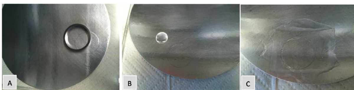
Figure B4: Grain mount preparation using epoxy as a base.
