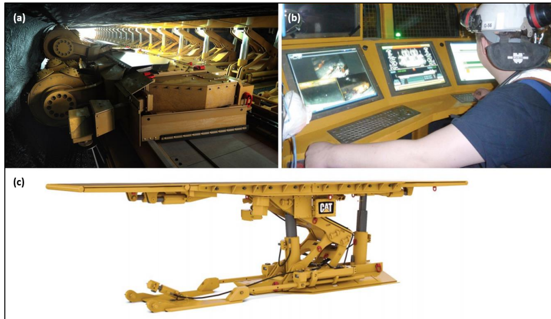
Figure 6.5 a) Caterpillar (CAT) Rock Straight System - underground hard rock narrow reef cutting machine b) Underground control room with an operator controlling the CAT rock straight system c) CAT Rock Straight Hydraulic roof support (Caterpillar, 2016)
