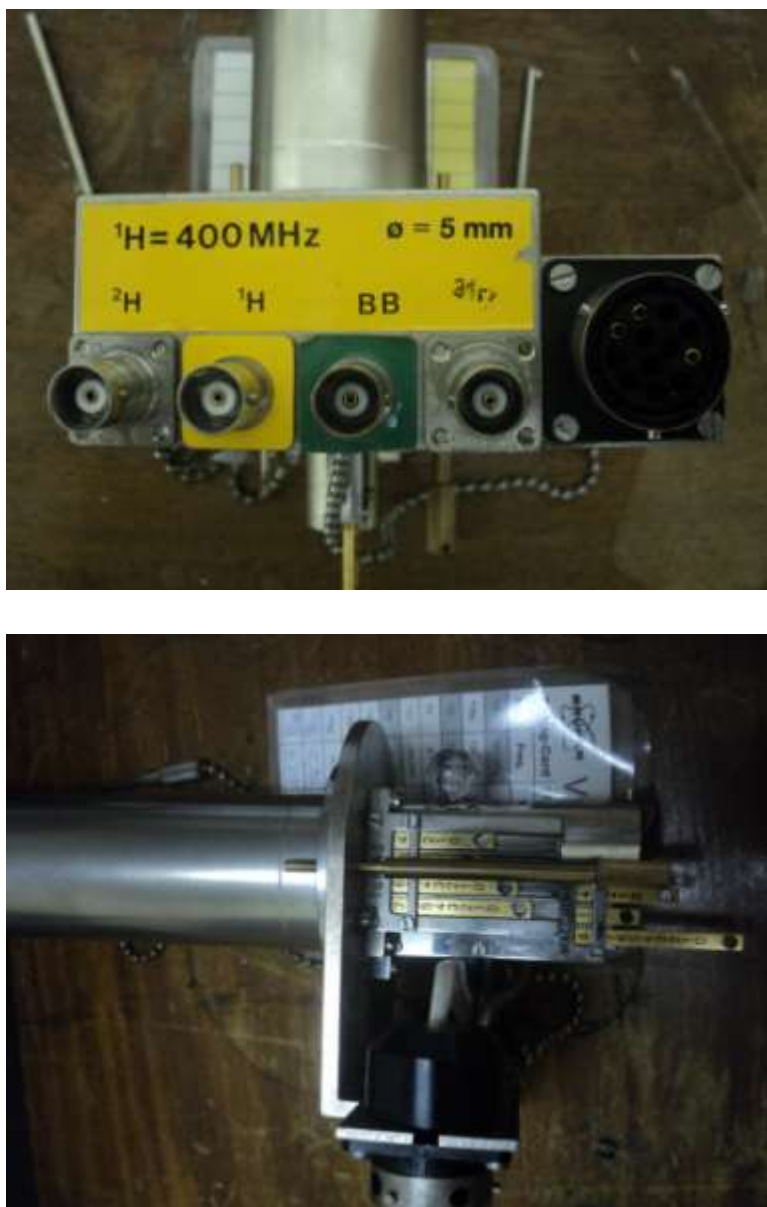
Figure 3.3 An image of a lower part of a 5 mm 400 MHz Bruker tripple resonance (TBI) probe
