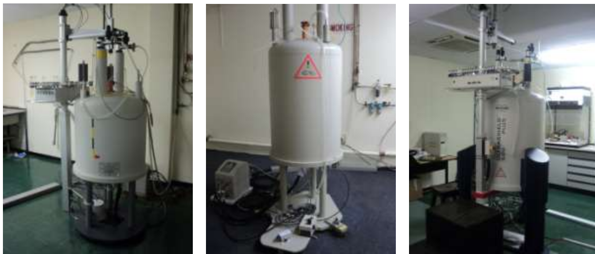
Figure 3.1 Three superconducting FT-NMR instruments used in the research (300, 400 and 500 NMR spectrometers)
