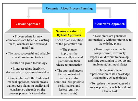
**Figure B.1** CAPP classification: The source of the process plans was the key method of CAPP systems classification (Alting and Chang 1989, Zhang 1994, Hugh 1994, Cay and Chassapis 1997, and Rozenfeld and Kerry 1999)
