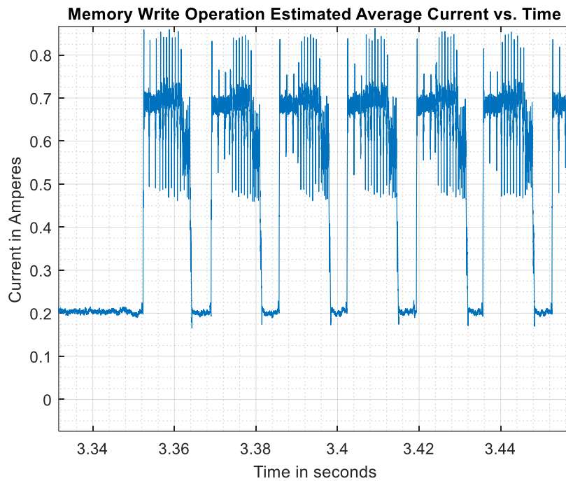
Figure 7.11: Zoomed-in estimated average current vs. time for memory write operation of the Cubieboard2
