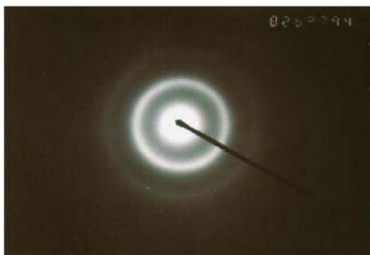
Figure 5 Selected-Area Electron Diffraction of an amorphous Ni-B alloy nanoparticles (Hoang & Ganguli 2012).
