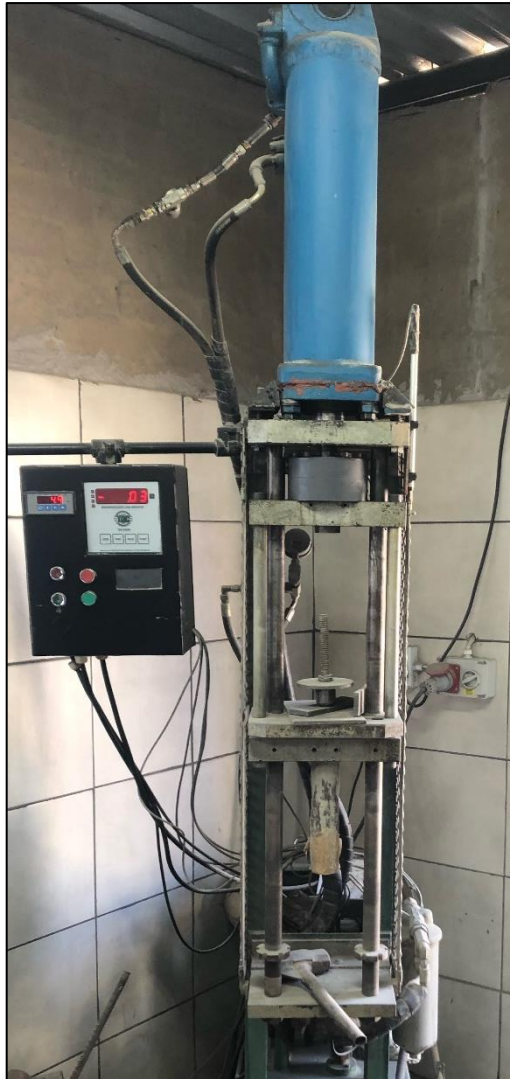
Figure 4.3-3. A picture of the 25-tonne pull-out testing bench.
