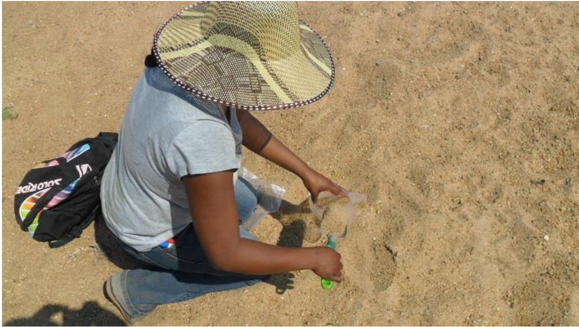
Fig. 4.3: Image of top sediment being sampled into a plastic sampling bag.
