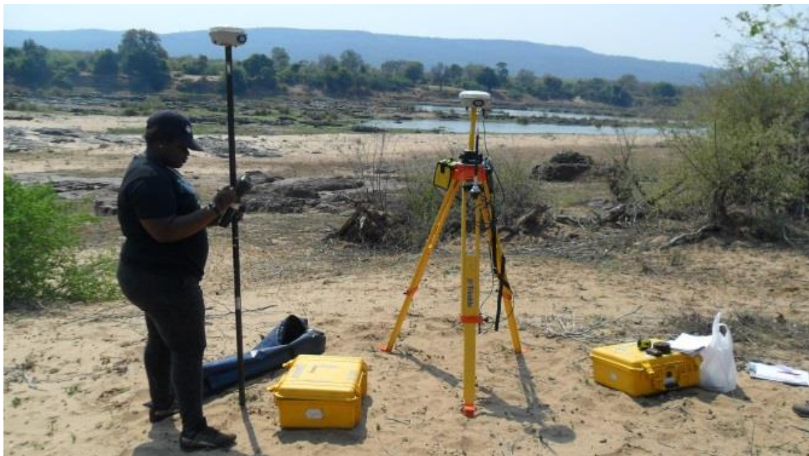
Fig. 4.2: Image of dGPS unit used to measure transects across the river channel.
