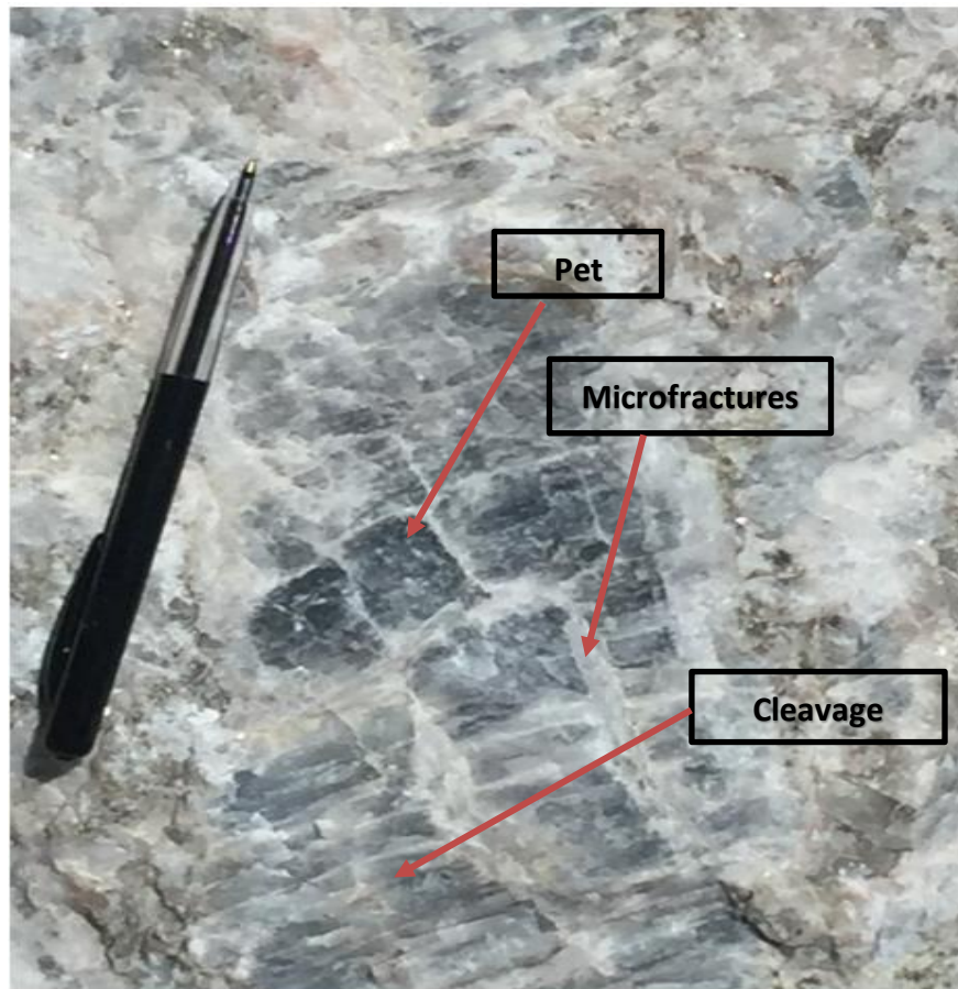
Figure 3. 7: Pit sample PS1, showing coarse-grained subhedral, brecciated grey petalite, with prominent microfractures and alteration along the cleavage planes (8034610N/331300E).
