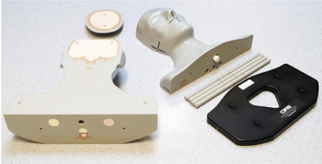
Figure 3.1 Different sections of the dismantled CIRS phantom (Model: 136500) showing the posterior, anterior and third small axial section. The base plate holder (black) is used to hold the sections together.
