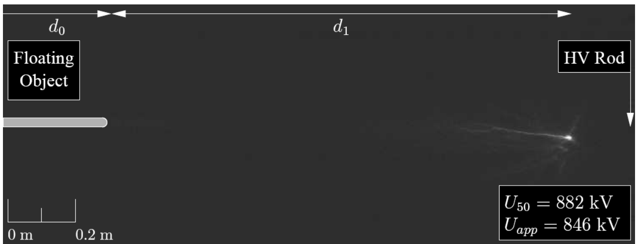
Fig. 6: High speed photograph of discharge occurring in the gap with the floating object at 50% from HV electrode resulting from a 25 \mu\text{s} applied impulse and 50 \mu\text{s} exposure time.
