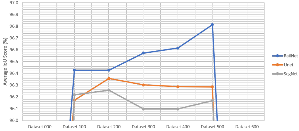
Figure 5.3: A focused comparison of RailNet, UNet and SegNet on each dataset
