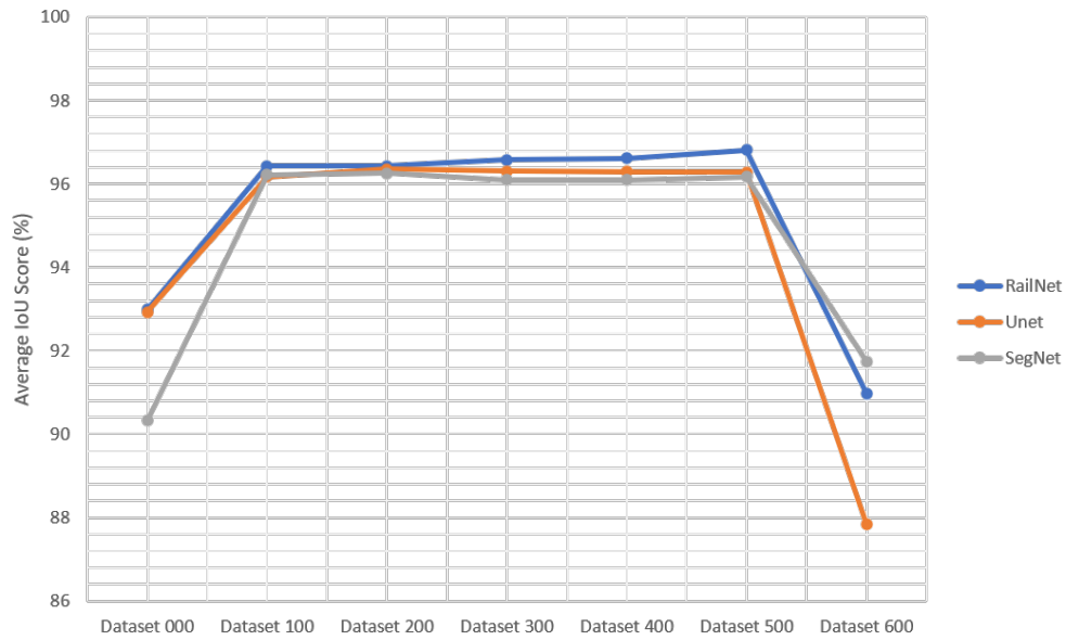
Figure 5.2: Comparison of RailNet, UNet and SegNet on each dataset
