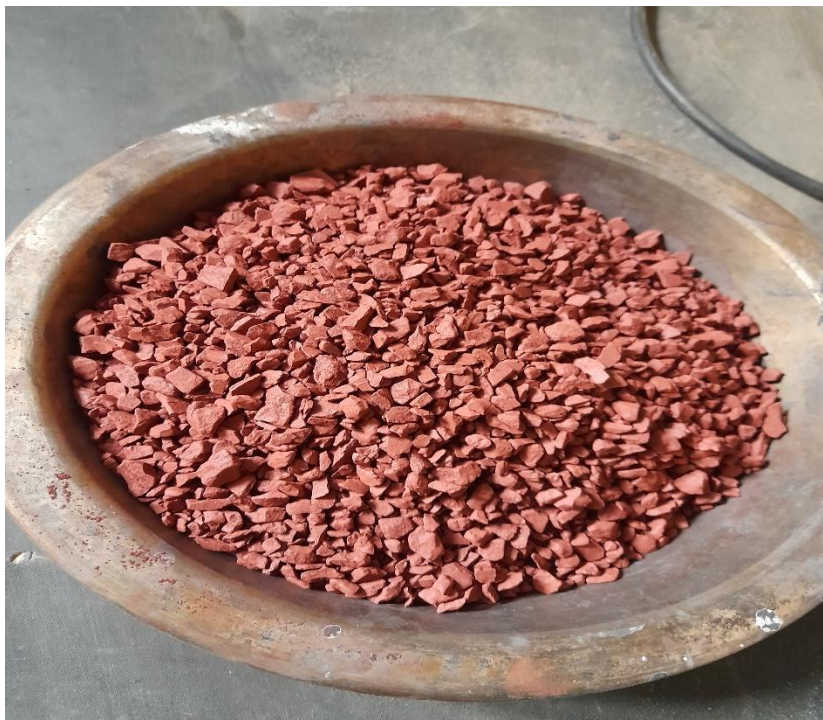
Figure 5: Photograph of a Hematite subsample after screening.
