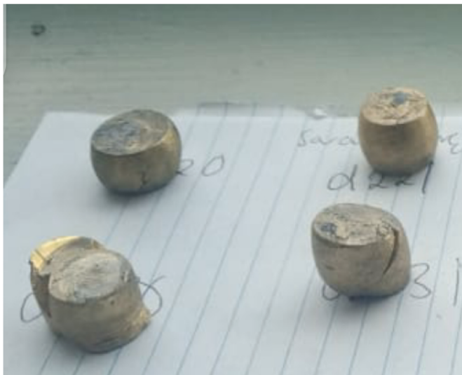
Fig. 6. Photograph of the hot deformed samples at 250 °C showing shearing-type deformation.
