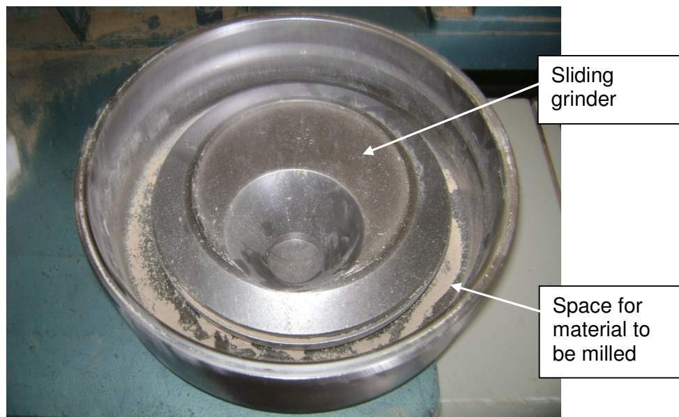
Figure 4.2 Swing mill pot opened to show the sliding grinder
