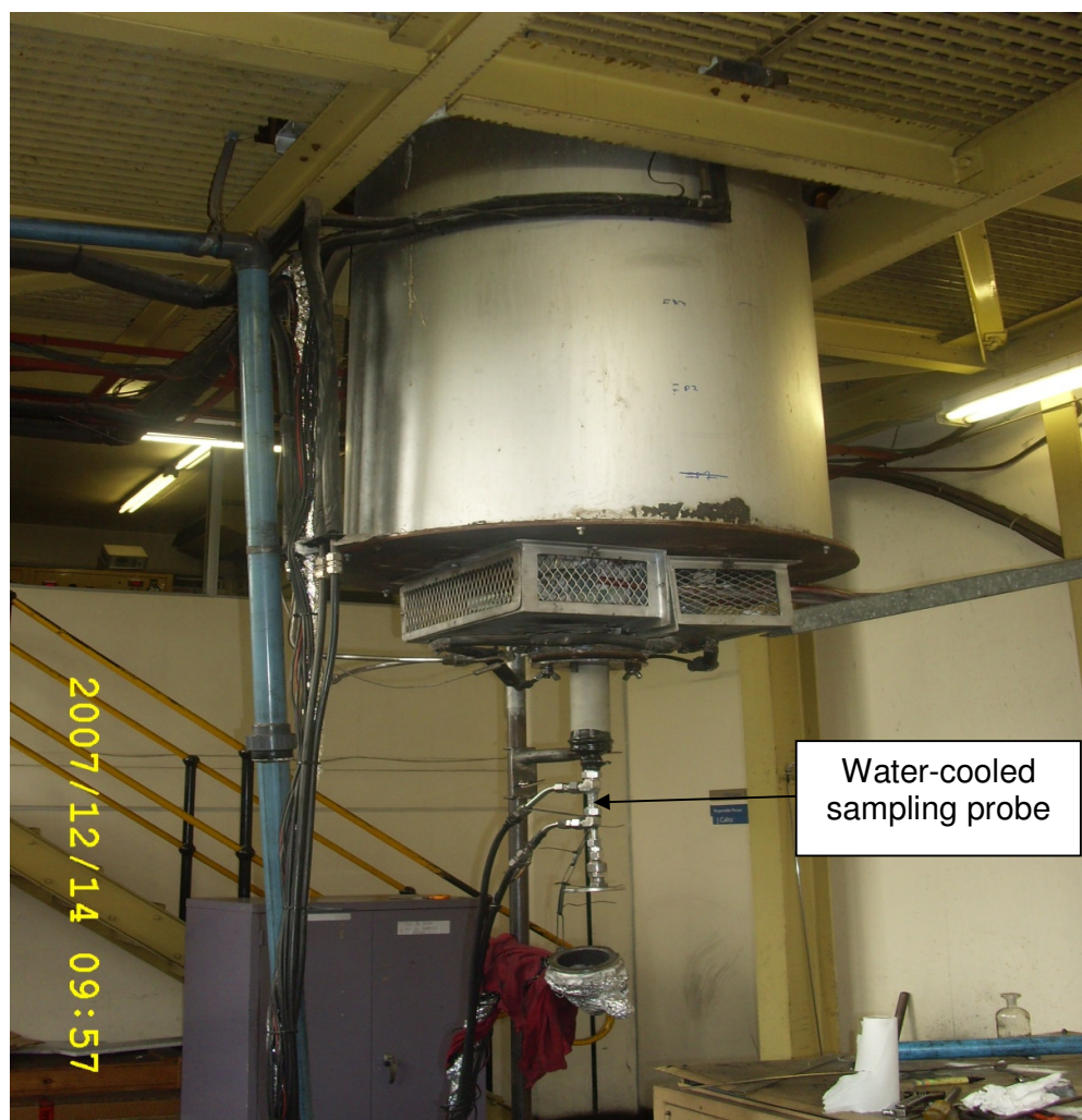
Figure 4.12 Eskom DTF Showing bottom-half with water cooled sampling probe
