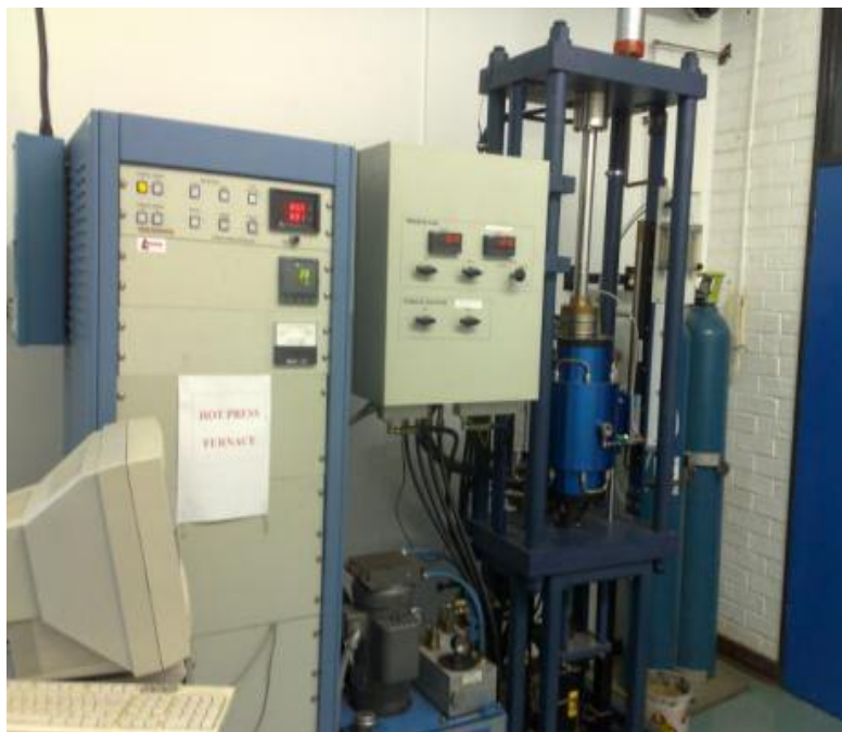
Figure 3.5: Uniaxial hot press
