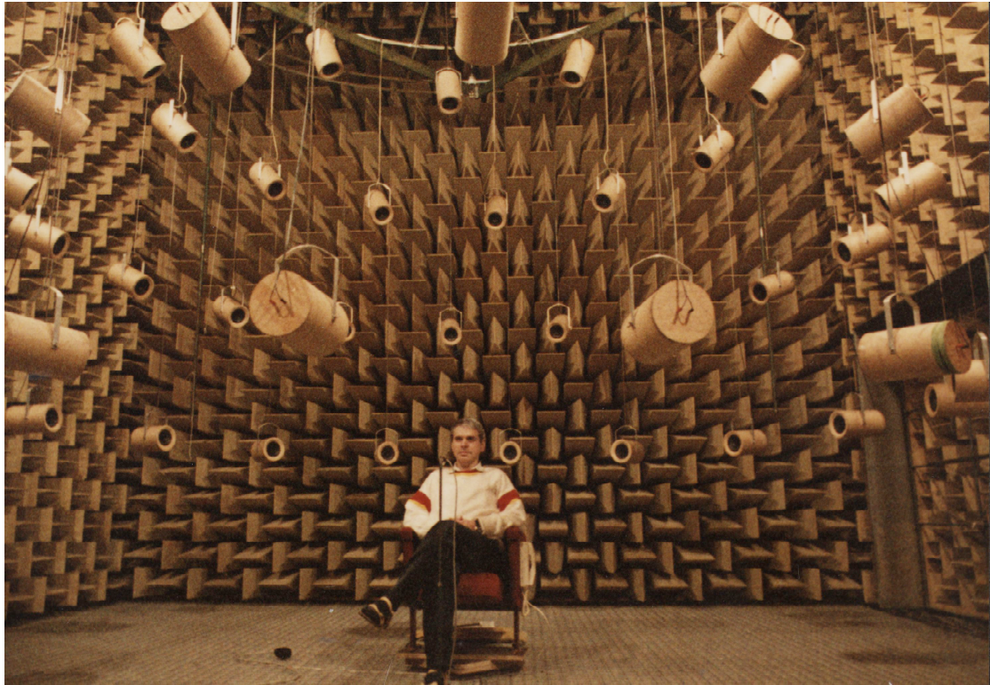
10. Prof. Mendel Kleiner listening to the hemispherical loudspeaker array used for auralization in the anechoic chamber. (1974)
