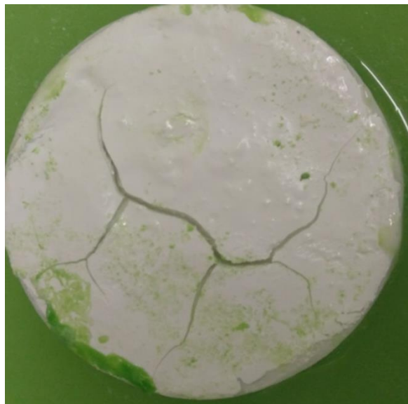
Figure 4-14: Cracks initiated due to fast drying as an effect of acetone.
