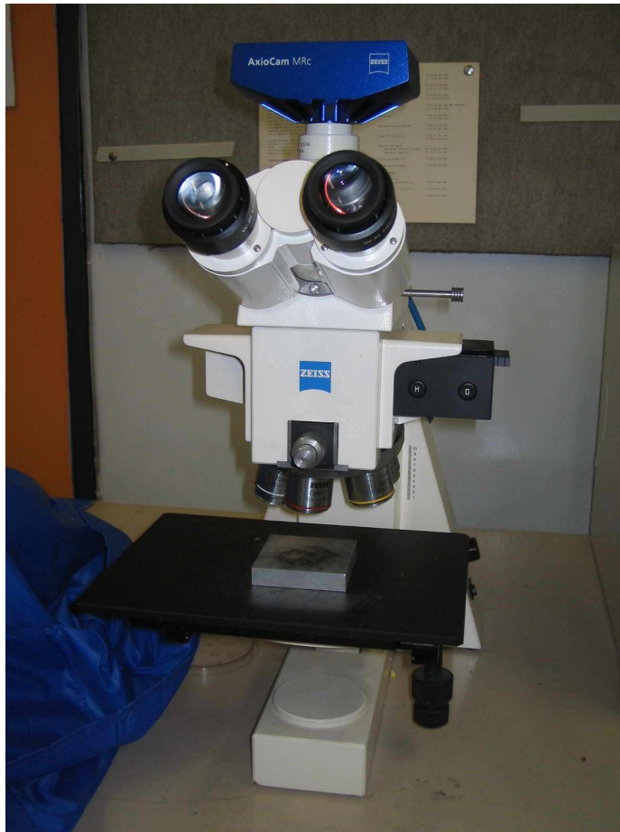
Fig. 3.3: The reflected light microscope used in this project
