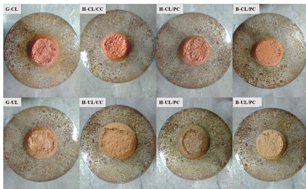
Figure 5.4: Images of spread diameter of the mortars.
