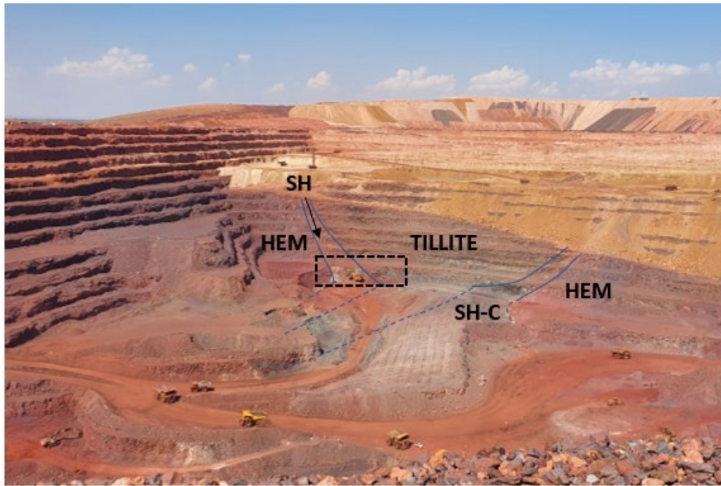
Figure 3.1: In-pit expression of carbonaceous shale (SH-C) at the Iron Ore Mine A
