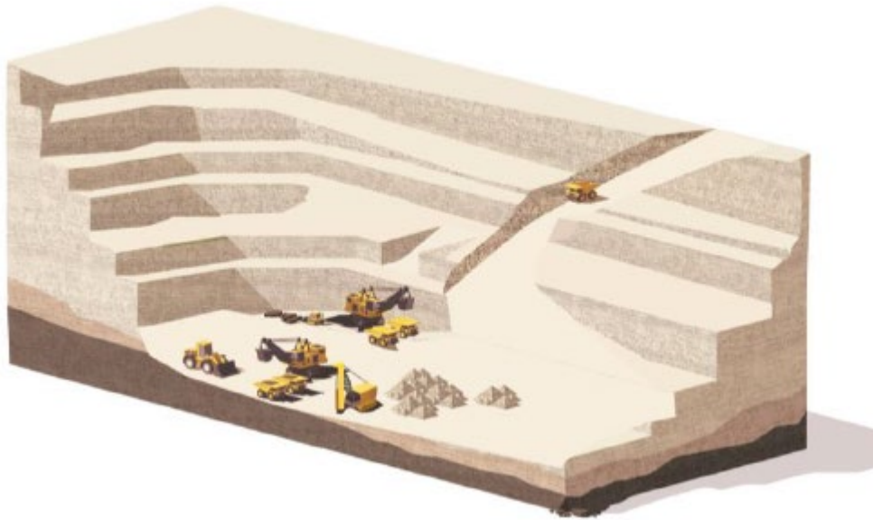
Figure 1.2: Conventional truck and shovel open-pit mining schematic (Anglo American, 2021)
