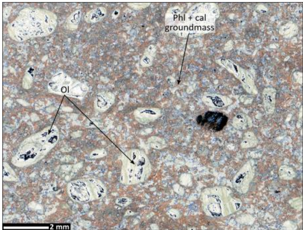
Figure 5.4. A photomicrograph scan of sample 41-166 showing serpentinised olivine macrocrysts set in groundmass composed of fine-grained (<1 mm) phlogopite and interstitial calcite. Ol- olivine, Phl- phlogopite and Cal- calcite (Whitney and Evans, 2010).
