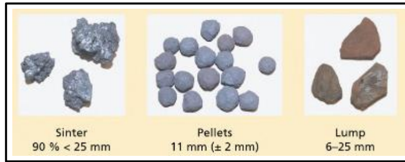
Figure 2.4 Forms of iron ore used in the blast furnace (Geerdes et al. , 2015)
